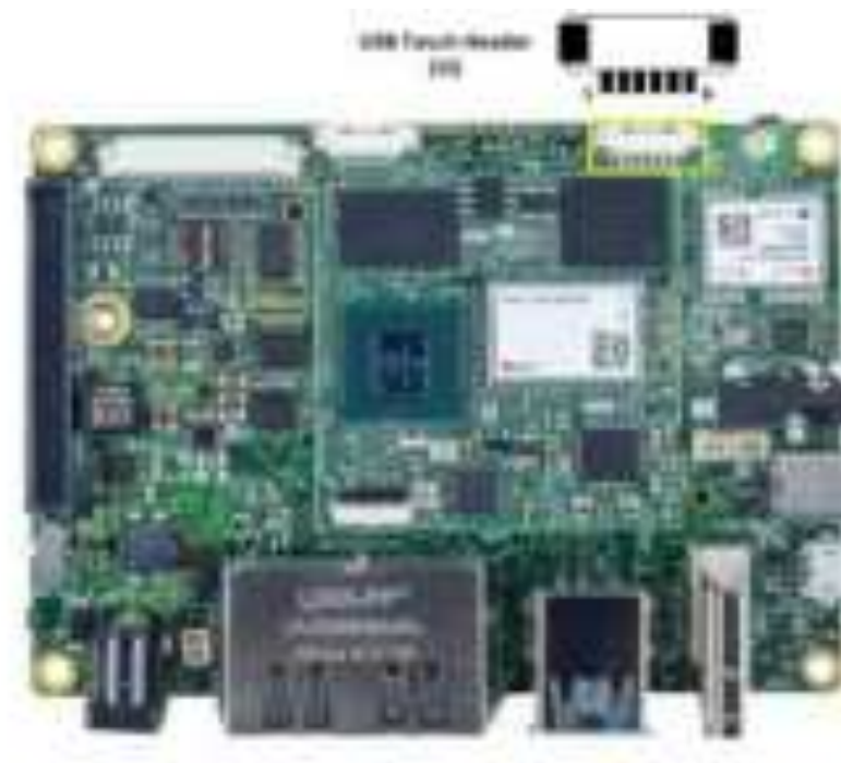
Figure 19: USB Touch Connector
