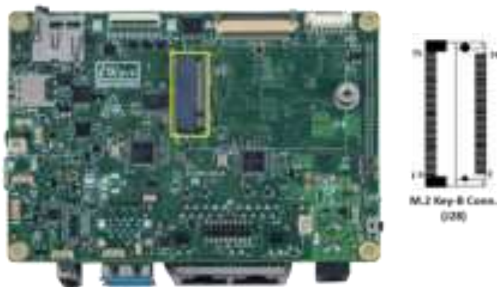
Figure 22: M.2 Key B Connector
