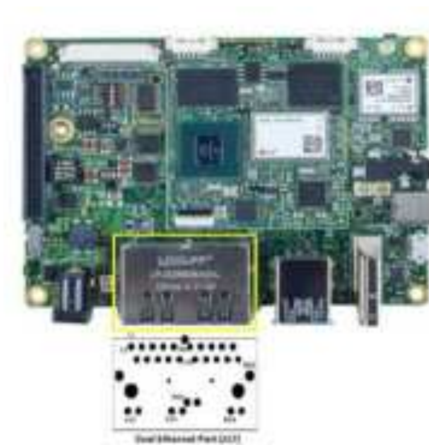
Figure 6: Dual RJ45 Magjack
