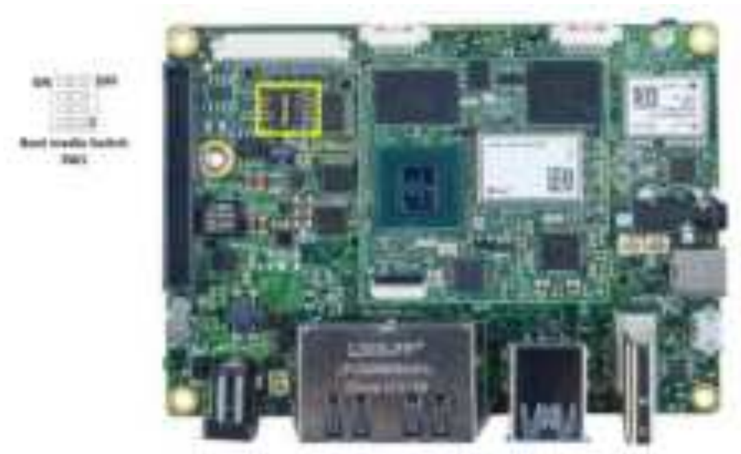
Figure 4: Boot Media Switch
