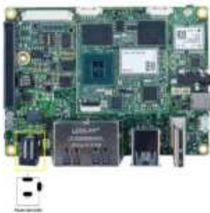
Figure 32: Power Input Jack
